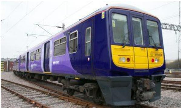
With the slow and expensive progression of electrification across the rail network, the suggestion of bi-mode trains has been introduced, using underfloor diesel power, but able to switch to electric power currently between Ely and Cambridge. An example of such a train is seen here to the left.
